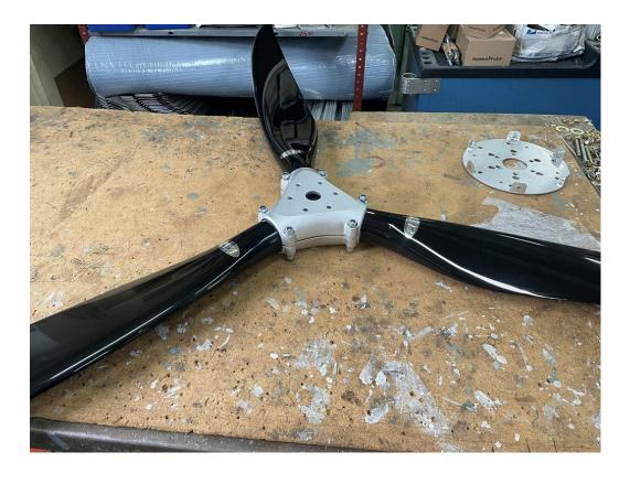
2. Make sure "0" marks on the propeller hub halves are aligned. Do not tighten the blade fixation bolts.
