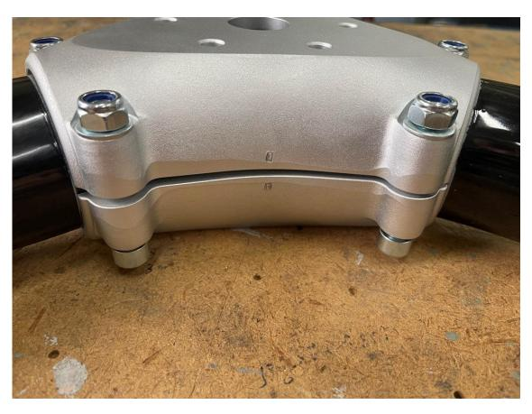
3. Install the propeller with the spinner base plate on the engine flange.
