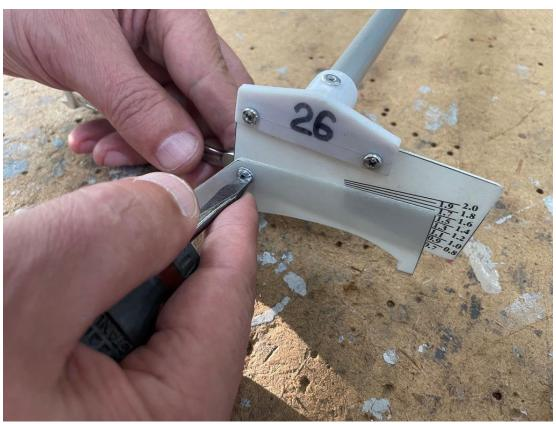
6. By lightly hitting the surface of the blade near its trailing edge, set the required pitch. When checking the pitch, the gauge should be based on the front face of the hub while the movable plate of the gauge should touch the surface of the blade without effort. The gaps at the points of contact of the gauge and the blade surface are not allowed.
