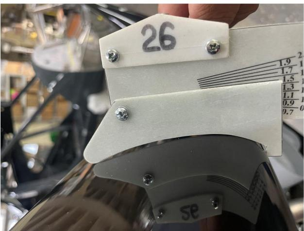
7. Tighten the fixation bolts of the blade adjusted to the required pitch with 10 N·m torque.
