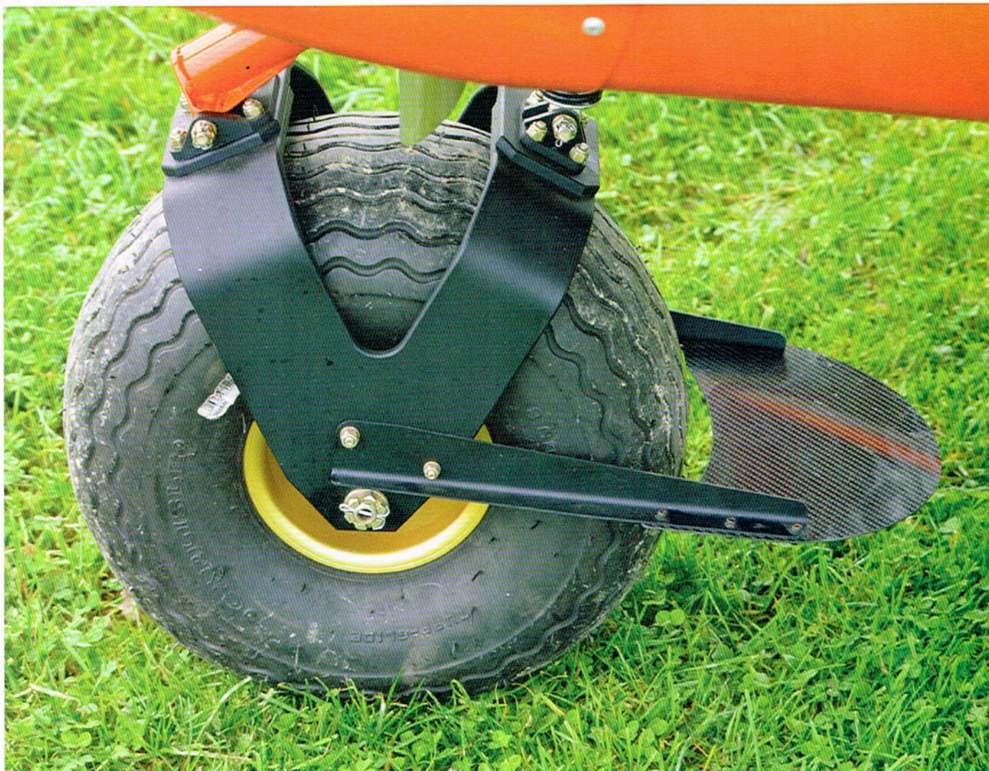
(Above) The neat mud/stoneguard on the Foxbat's chunky nosewheel reduces the amount of grime accrued and also any potential stone damage to the underside of the fuselage. (Photo: John Macknay)
