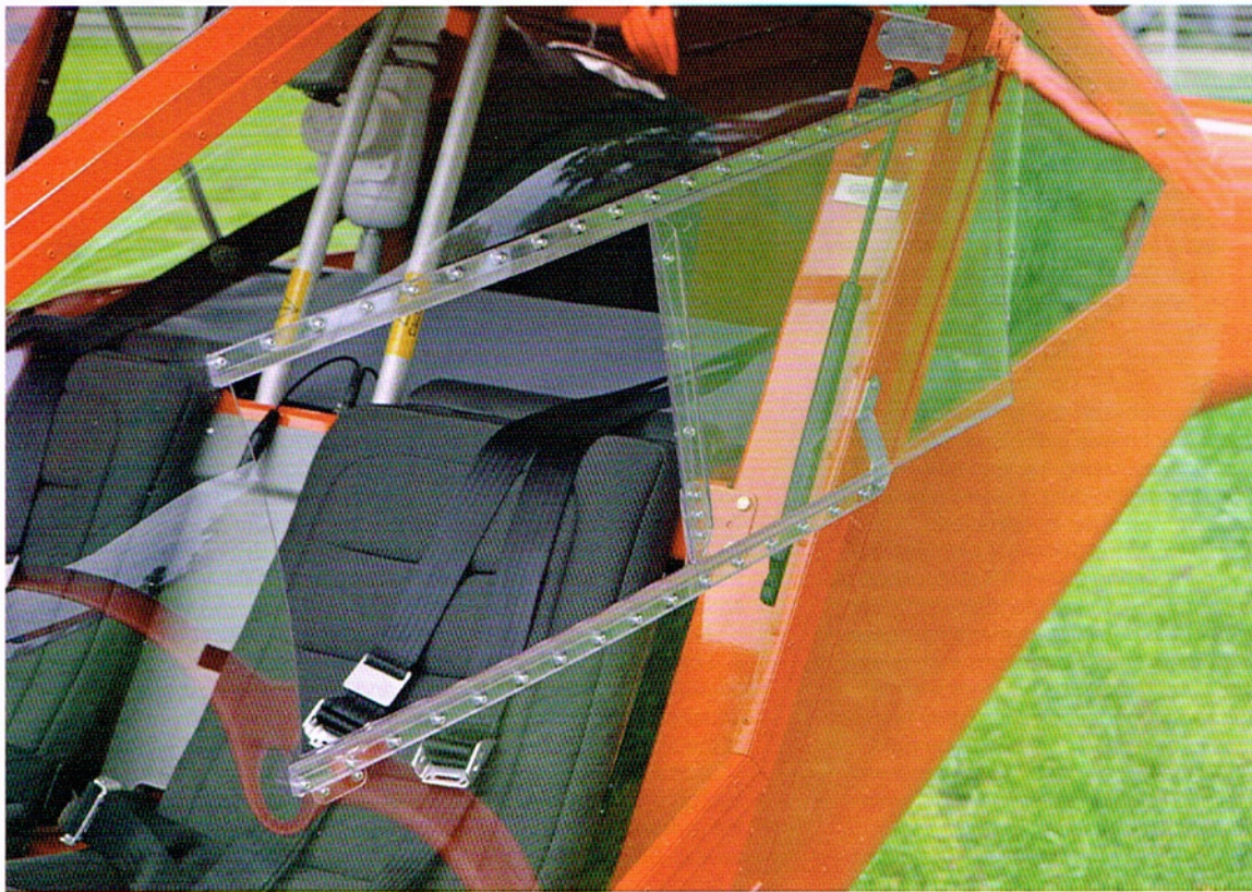
(Left) The large camera aperture/clear-view panel in pilot's door. (Photo: John Macknay)
